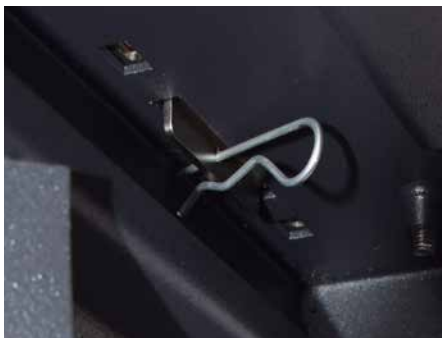
7. Secure the glass hood from below with the 4 glass retaining clips as shown.
