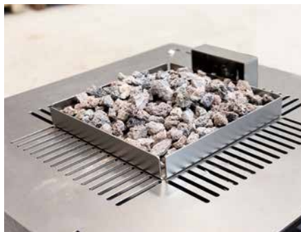
5. Spread the lava stones in the form of a small hill on the burner bed. Make sure that no small stone chips get into the burner.
